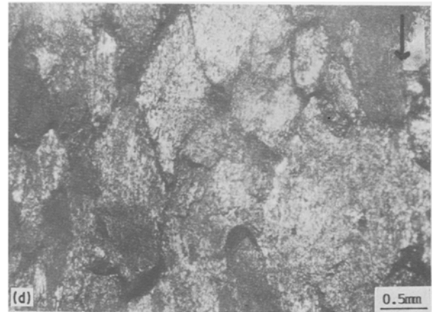
Figure 4 Metallographic observation of cyclically crept specimens. (a, b) Peak stress 15 MPa, stress frequency 3 cycles per minute, stress amplitude 90%; (c) cyclic creep after electropolishing and surface marking, same stress conditions as (a); (d) Statically crept specimen, stress 15 MPa. Arrows indicate the stress axis.
